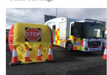
Kier is trialling inflatable safety barriers that can be put up in a matter of minutes to help protect road workers.
